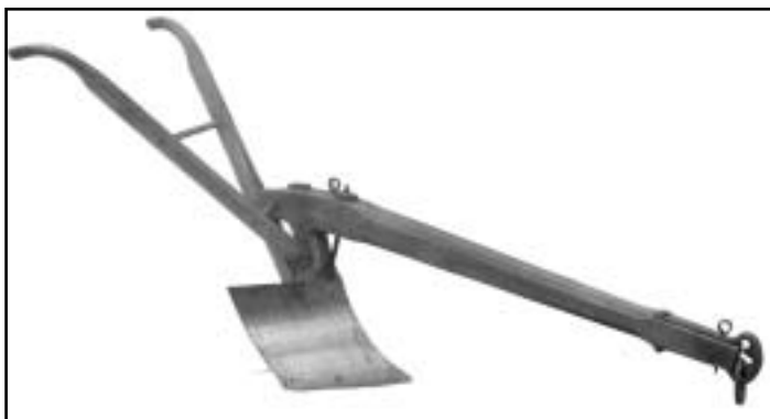
The first steel-faced plow was invented by John Deere in 1837 at his blacksmith shop in Grand Detour, Illinois. This self-scouring steel plow did a better job cutting through the tough prairie sod than wooden or cast iron plows. Illustration courtesy of the Illinois State Historical Library.
